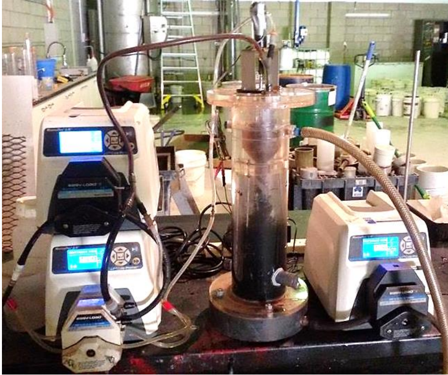
Figure 5: - 99 mm Diameter Lab Scale Thickener used for laboratory dynamic thickener test work.
