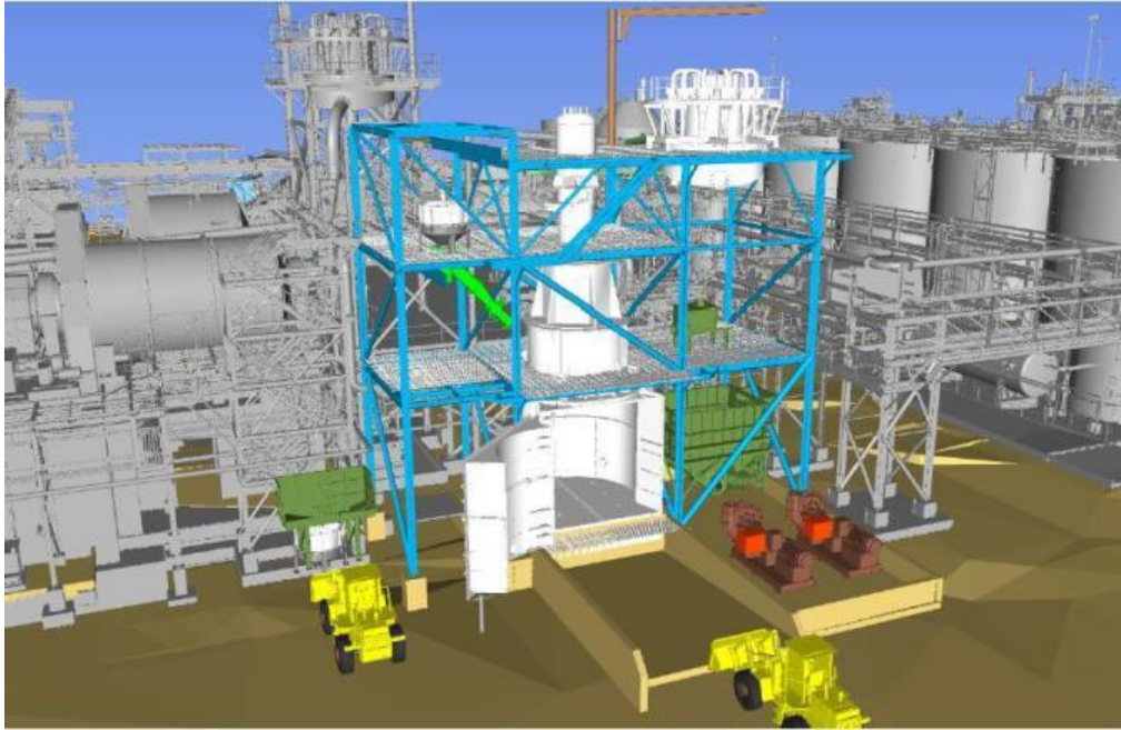
Figure 8 - General Arrangement of Vertimill Circuit
