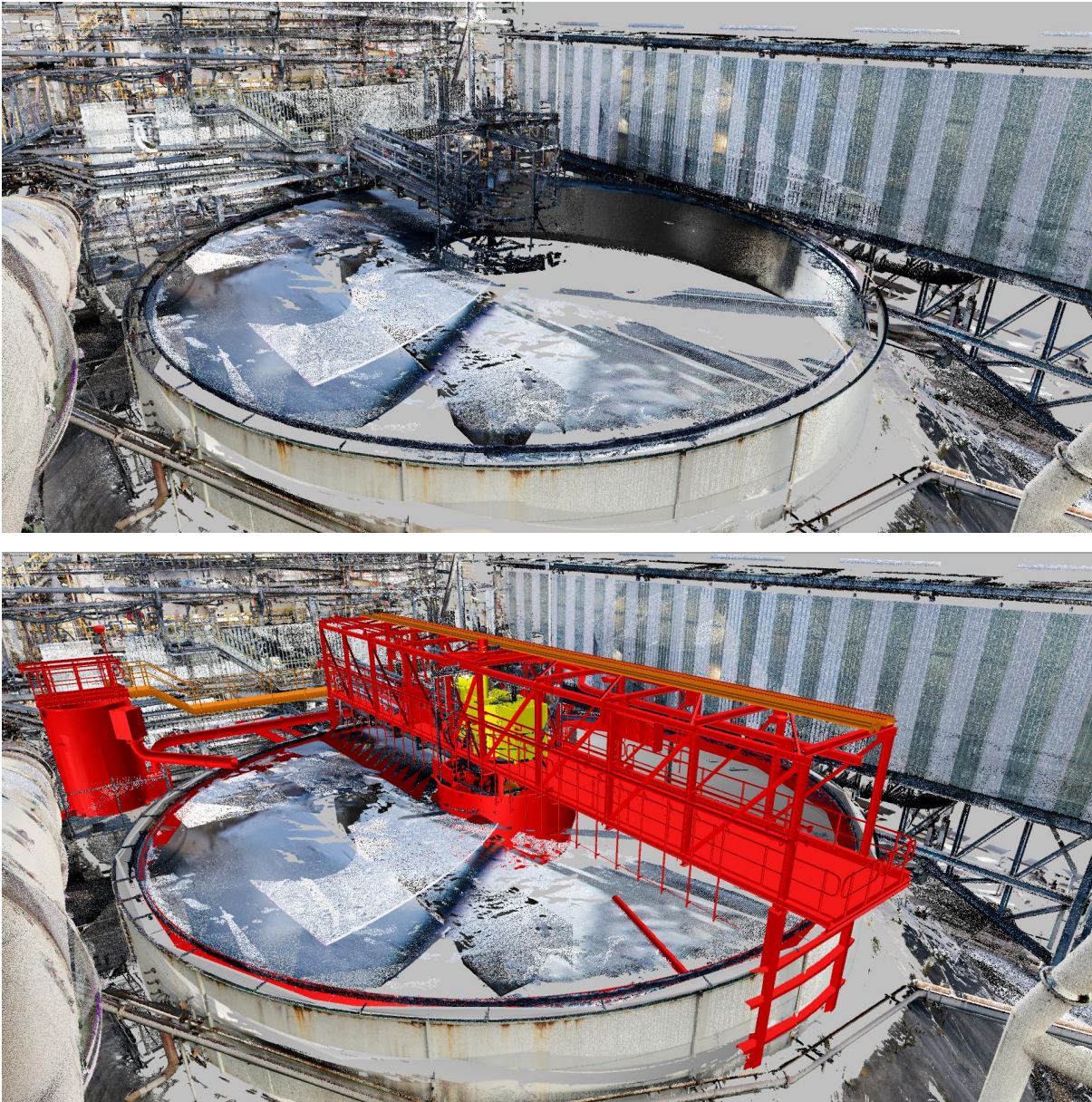
Figure 11: Laser scan images showing before upgrade arrangement versus final upgrade design models.
