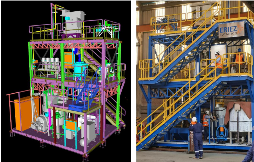
Figure 7 HydroFloat CPF Pilot Test work Unit (courtesy of Eriez)
