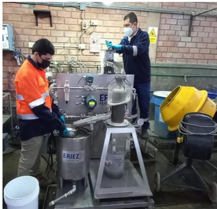
Figure 6 HydroFloat CPF Lab Test work Unit (courtesy of Eriez)
