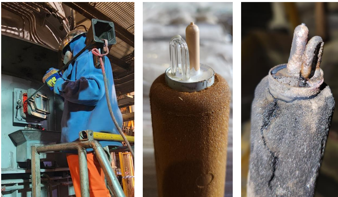
Figure 9 - Uptake shaft temperature and oxygen measurement & celox probe before & after
