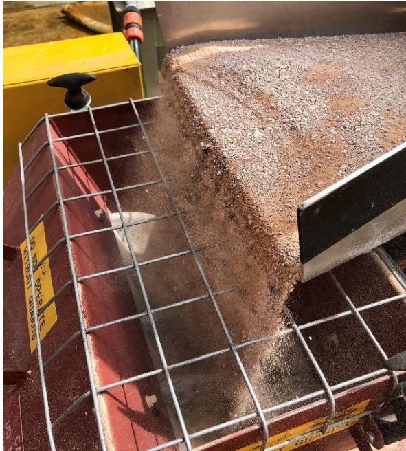
Figure 15: GRolls Dry – 3 mm limestone feed material
