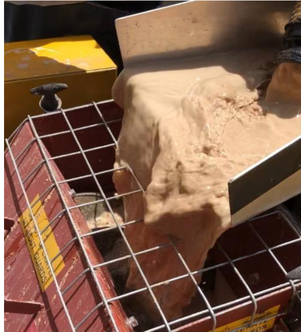
Figure 16: GRolls Wet 33% solids (w/w) slurry – 3 mm limestone feed material
