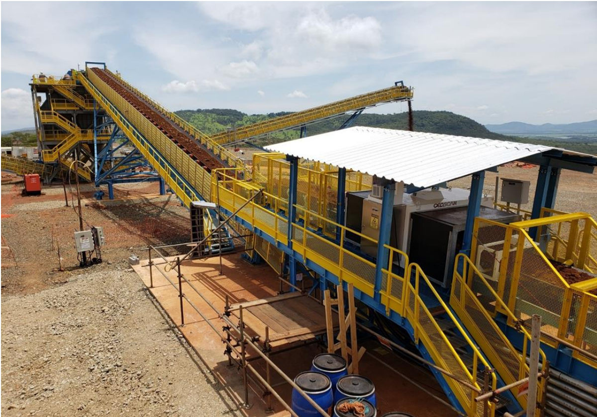
Figure 4 – High specification GEOSCAN analyser generating representative, multi-elemental data used in a base metals bulk ore sorting plant for 30 second parcel diversion.
