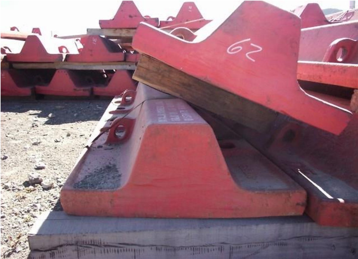
Figure 2: the first top hat, or sombrero, SAG shell liners, Alumbreira, Argentina, 1997
