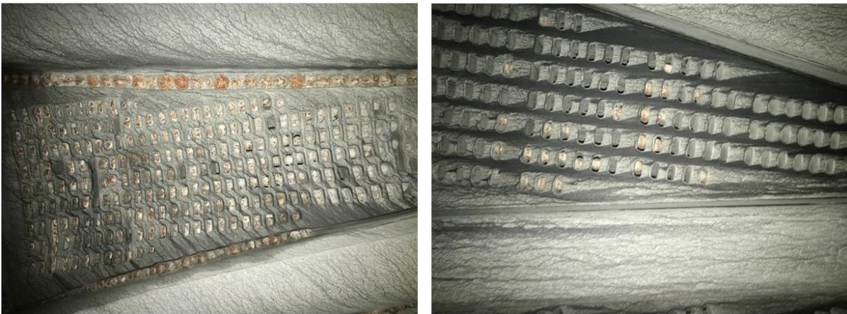
Figure 7: Comparison between original grates (left) and modified design (right) after similar operating hours.
