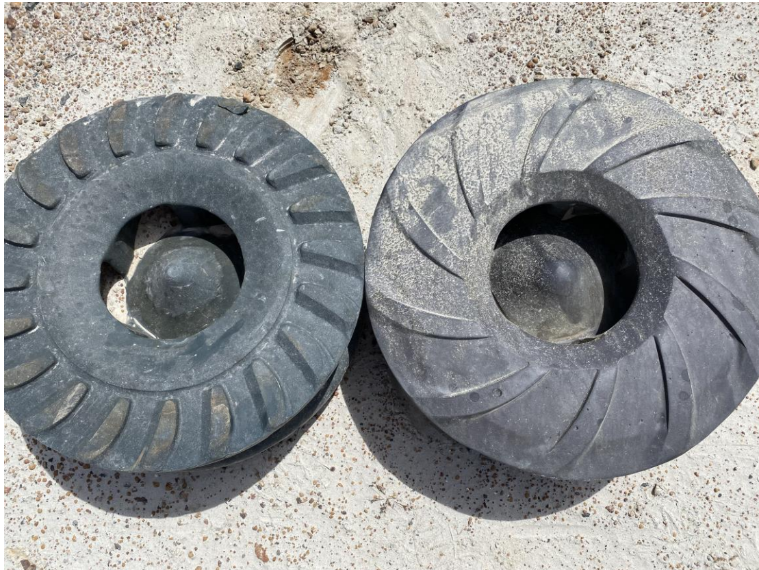
Figure 8. Two impellers for the same pump with claimed equivalent performance.
