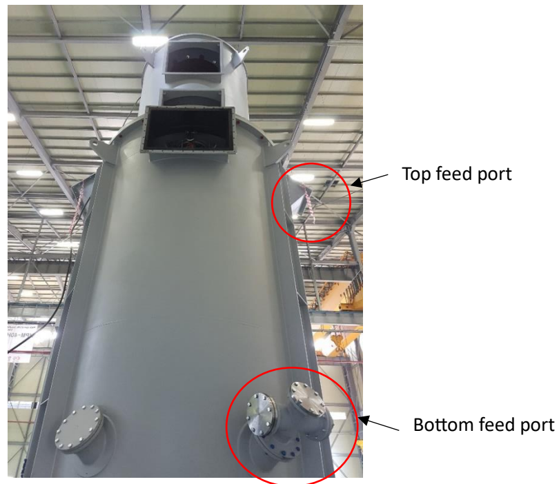
Figure 8: Mill feed configuration – top and bottom
