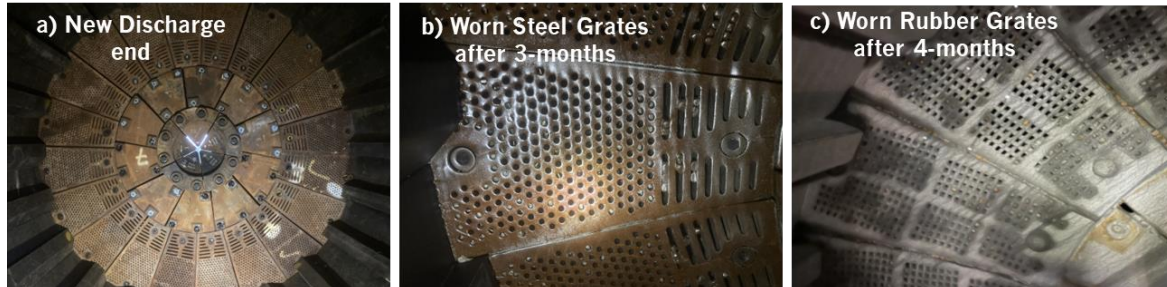
Figure 11: a) Mill#2 with grate-EEPL discharge end and b) worn steel grates after 3 months c) worn rubber grates after 4 months.
