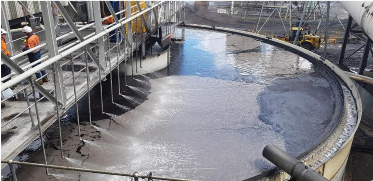
Figure 13: Thickener operating after upgrade, note overflow clarity and low levels of froth on thickener surface.
