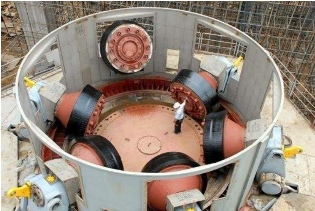
Figure 2. Internal view of a VRM for approximately a 1000 t/h duty (Image courtesy of Mining Technology, 2023)
