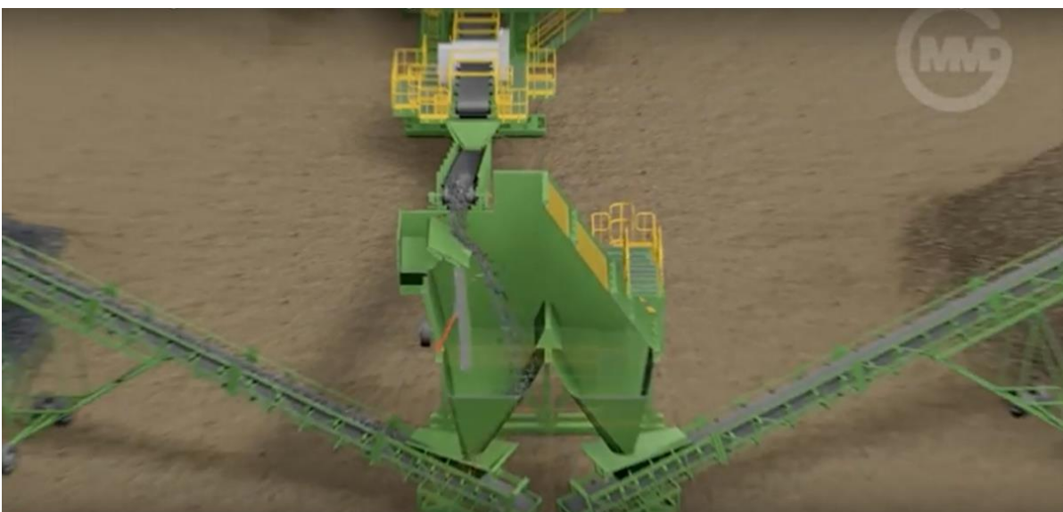
Figure 5 – Example of a diversion system used in a copper ore bulk sorting plant for ore flows of 500 t/h (Hillyer, 2019)
