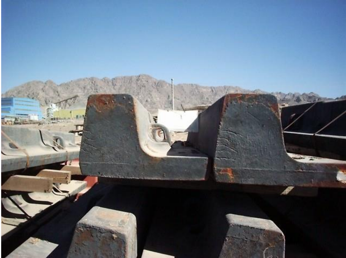
Figure 1: the typical 1990s rail bar SAG shell liner
